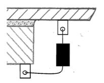
Typical installation of Spark Gap EX-FS-KU
